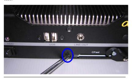
Step 10: Close the rear case of AEC-6523 and fasten the two screws on the rear case.
