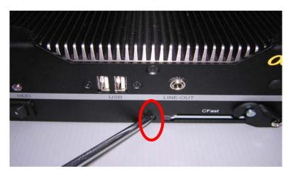
Step 4: Loosen the screws on the rear panel of AEC-6523
