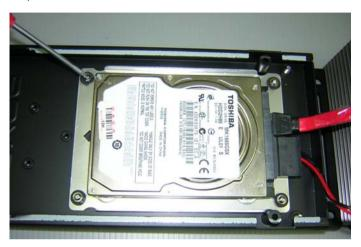
Step 8: Fasten the bottom HDD kit case of AEC-6523.
