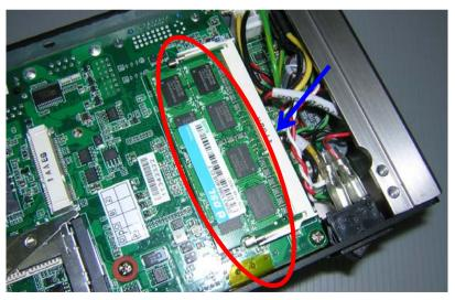
Step 7: Adhere the heat-spreading sheet to the SDRAM.
