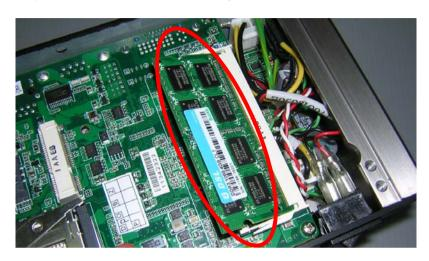
Step 6: Press the SDRAM and make sure that it has been inserted properly.
