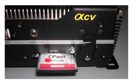
Step 4: Fasten the cover of the CFast™ card.
