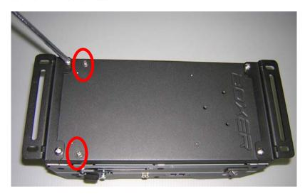
Step 9: Close the front case of AEC-6523 and fasten the screw on the front case.
